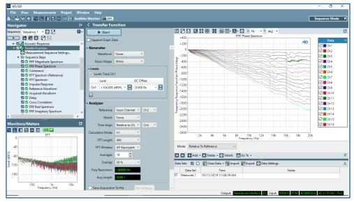
PDM 16 Phase Spectrum Measurement in APx500 Software
